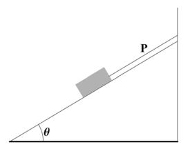
**Solution** : Since the block is moving at constant speed up the incline, the sum of all forces up the incline must sum to zero. Our force equations become :
