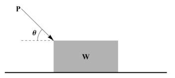
**Solution :** Again we sum forces in the horizontal and vertical directions. Since the block has yet to move, we use the coefficient of static friction. Note : because there is a component of P that acts vertically, the normal force will not equal the weight of the crate. Many students made this error.
