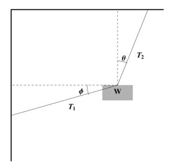
**Solution** : Since the system is in equilibrium, all the horizontal forces sum to zero, and all the vertical forces sum to zero. (Notice that the vertical component of  $T_1$  acts down.) This means that :
