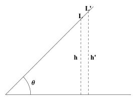
Let's say the mass encounters the spring when it has traveled L units along the ramp (and is h units high), and has traveled L' units when it fully compresses the spring (and is h' units high). The mass compresses the spring by an amount (L'-L); in moving from L to L', the mass gains m g (h'-h) in gravitational potential energy. Using the diagram we can see that this increase in GPE is simply m g(L'-L) sin  $\theta$ .
