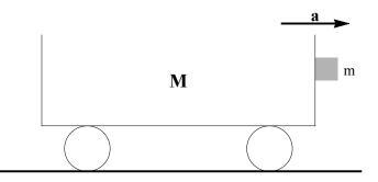
**Solution**: The only horizontal force acting on m is the normal force due to contact with M. Since m is acceleration at a, we can write that N = m a. The box will not slide down if the force of static friction equals the weight of m. This condition can be written as:
