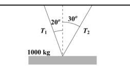
We first delineate the forces acting on the beam. These are the weight of the beam, and the tension in the two ropes. The weight acts down, and each tension has both a vertical and horizontal component. Newton's second law gives :
