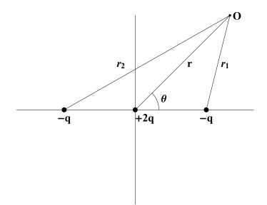
The -q charges are located at (a,0) and (-a,0) along the x-axis. Express the potential at O due to this arrangement of charges in terms of Legendre polynomials. Assuming a<<r, what is the leading term of the expansion?
