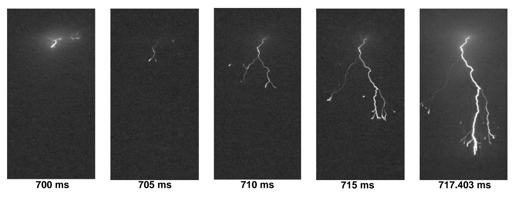
**Figure 3**: Lightning images captured by Phantom v2012 high speed video camera from start of event to return stroke.
