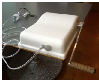
The Human-Powered Nebulizer (HPN) gets its power from a hand crank on the side of the device. Just like any other nebulizer, the HPN converts liquid medicine into a mist that can be inhaled deep into the lungs.
