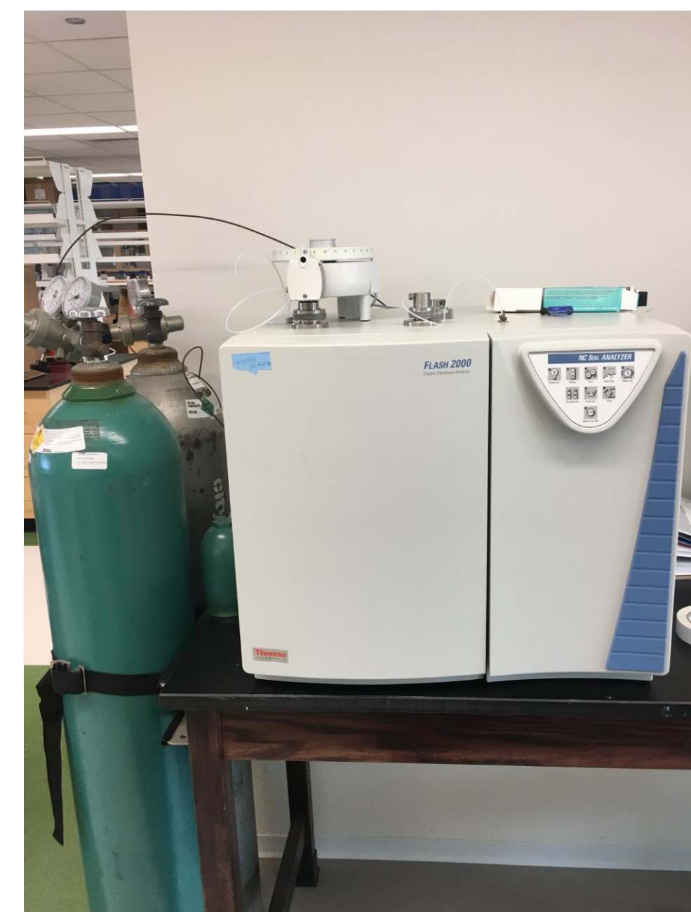
Image 4: Flash 2000 Organic Elemental Analyzer for protein content analysis.
