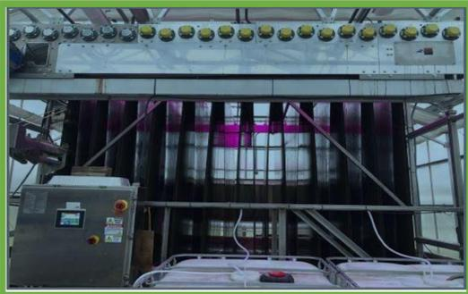
Figure 1. Algae grow on vertical 10-ft. belt at the O'Brien Water Reclamation plant in Skokie, Illinois.
